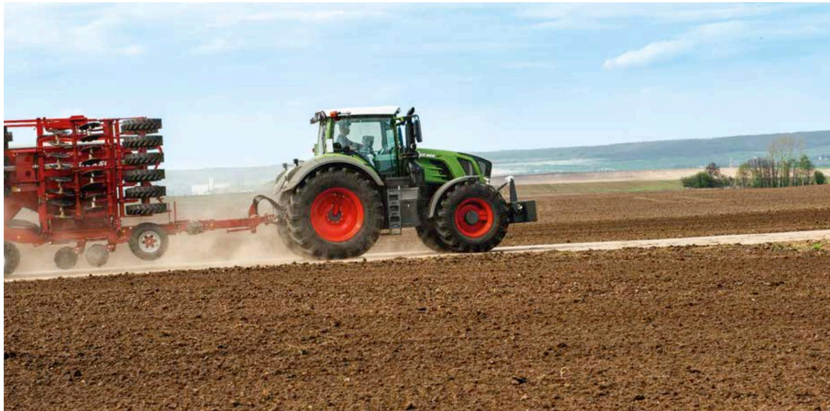
The Fendt 800 Vario has a self-levelling front axle suspension as standard. It has a 120-mm suspension travel, plenty to level uneven surfaces. The  $\pm 8^\circ$  swing angle ensures stability while driving. The  $50^\circ$  maximum steering angle on the front axle guarantees maximum manoeuvrability. The entire suspension travel can be run through manually when standing still, e.g. for picking up a front weight without front linkage.
