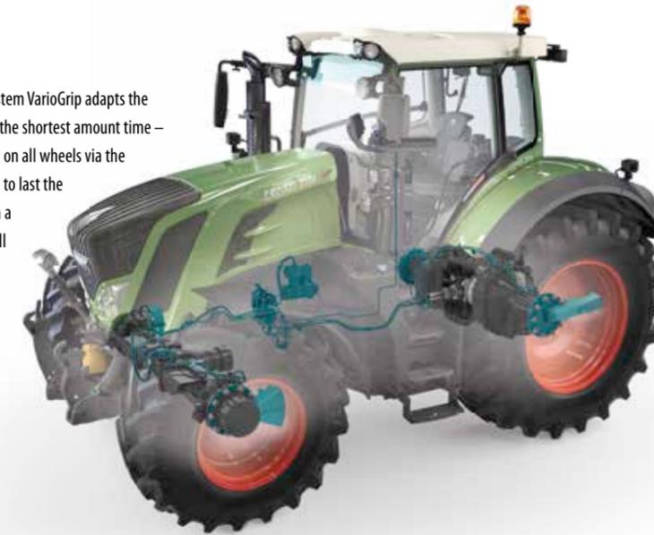
Using the Varioterminal, the tyre pressure of the tractor can be controlled with just a push of a button. The assistance system informs drivers about too low or too high tyre pressure.
