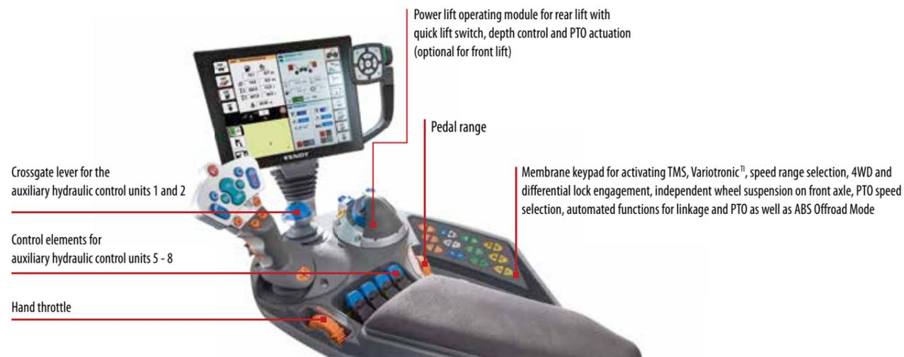
With Variotronic<sup>®</sup> headland management, operators can create operating sequences for turns, while driving or standing still, and save them. Settings for the engine and transmission control, the hydraulic valves and the front and rear linkage, the front and rear PTO as well as the automated steering system along with their individual functions are made via the headland management system and can be called up easily.
