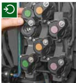
The double-sided CUP (couple-under-pressure) couplings make mounting and removing the implements much easier. The self-closing valve flaps effectively protect against contamination and permit one-handed connection of a hydraulic line.
