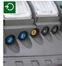
With the external valve controls, you can actuate the rear linkage, one valve and the PTO directly on the rear mudguard. Using the external controls for the rear PTO, a preset engine speed can be targeted automatically. You save yourself unnecessary steps, for example, when filling the slurry tank.
