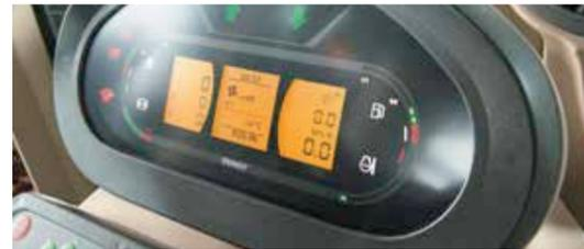
■ The interior lighting in the Fendt 800 Vario is perfectly designed for the important areas. Whether day or night, the most important operating elements are pleasantly backlit. The intensity of the backlighting is automatically controlled in the Varioterminal via a light sensor, dependent on the light conditions.
