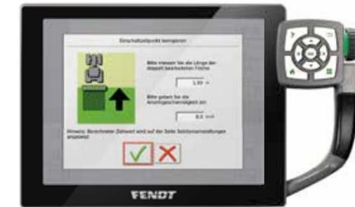
When operating ISOBUS-capable sprayers, fertiliser spreaders or seed drills, SectionControl can now switch up to 36 sections.
