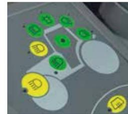
■ The lighting is easily set and adjusted thanks to its straightforward layout. With the smart one-button system, all previously set work lights can be switched on easily and quickly with just one touch of a button in the membrane keypad.
