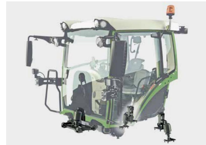
□ The cab suspension with air spring elements enables a fully vibration-minimised cab. The great difference in height and the long distance between the spring elements of the x5 cab also prevent bouncing and ensure maximum ride comfort.
