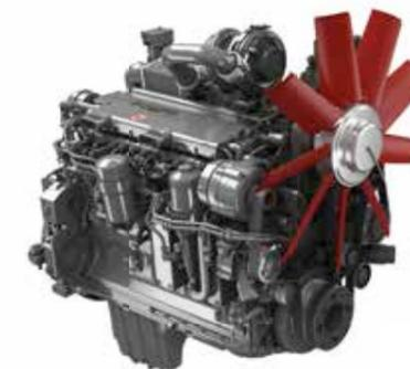
The reversible fan can automatically reverse the air flow so the radiator elements can be blown out effectively. What's special: Depending on the cooling requirement, the position of the fan blades is adjusted to achieve more efficient cooling. This has a positive impact on the fuel-efficiency.
