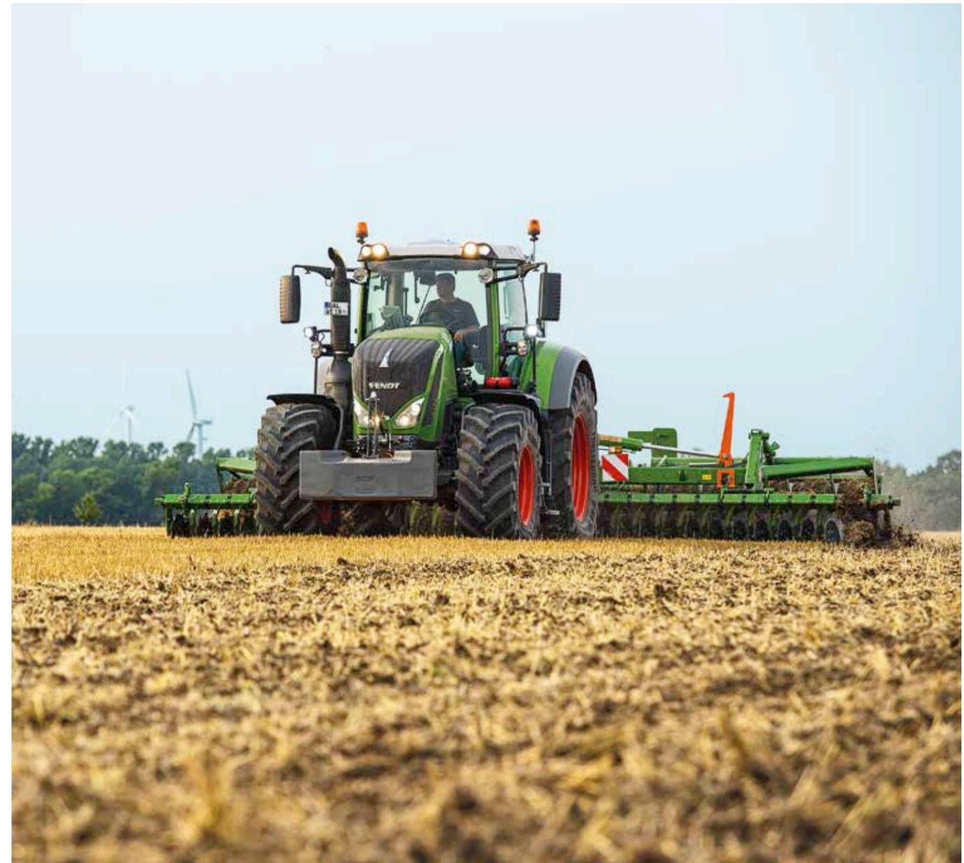
The tractor regulates the load limit fully automatically and adjusts the engine speed and transmission ratio. In this way, the engine and transmission are perfectly coordinated, which means extremely low fuel consumption.
