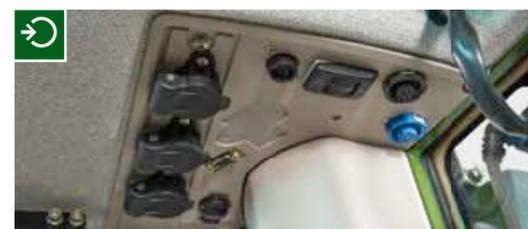
□ Numerous sockets are available in the cab, e.g. several 12-Volt sockets, ISOBUS socket, signal socket.
