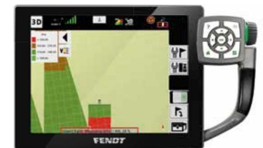
With VariableRateControl (VRC), you can farm according to site-specific application maps, depending on the ground and crop. So you can save on inputs.
