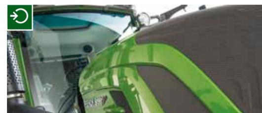
A special feature of a Fendt tractor is the standard specification bonded front windscreen. For even greater comfort and safety, a heated front windscreen made of laminated safety glass is also available.
