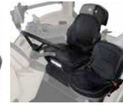
□ The air-suspended super comfort seat Evolution dynamic Dualmotion has an adaptive backrest, seat heater, low frequency suspension, pneumatic lumbar support and adjustable armrest. The seat cover is available in either a black fabric or black, smooth leather in combination with a leather steering wheel.
